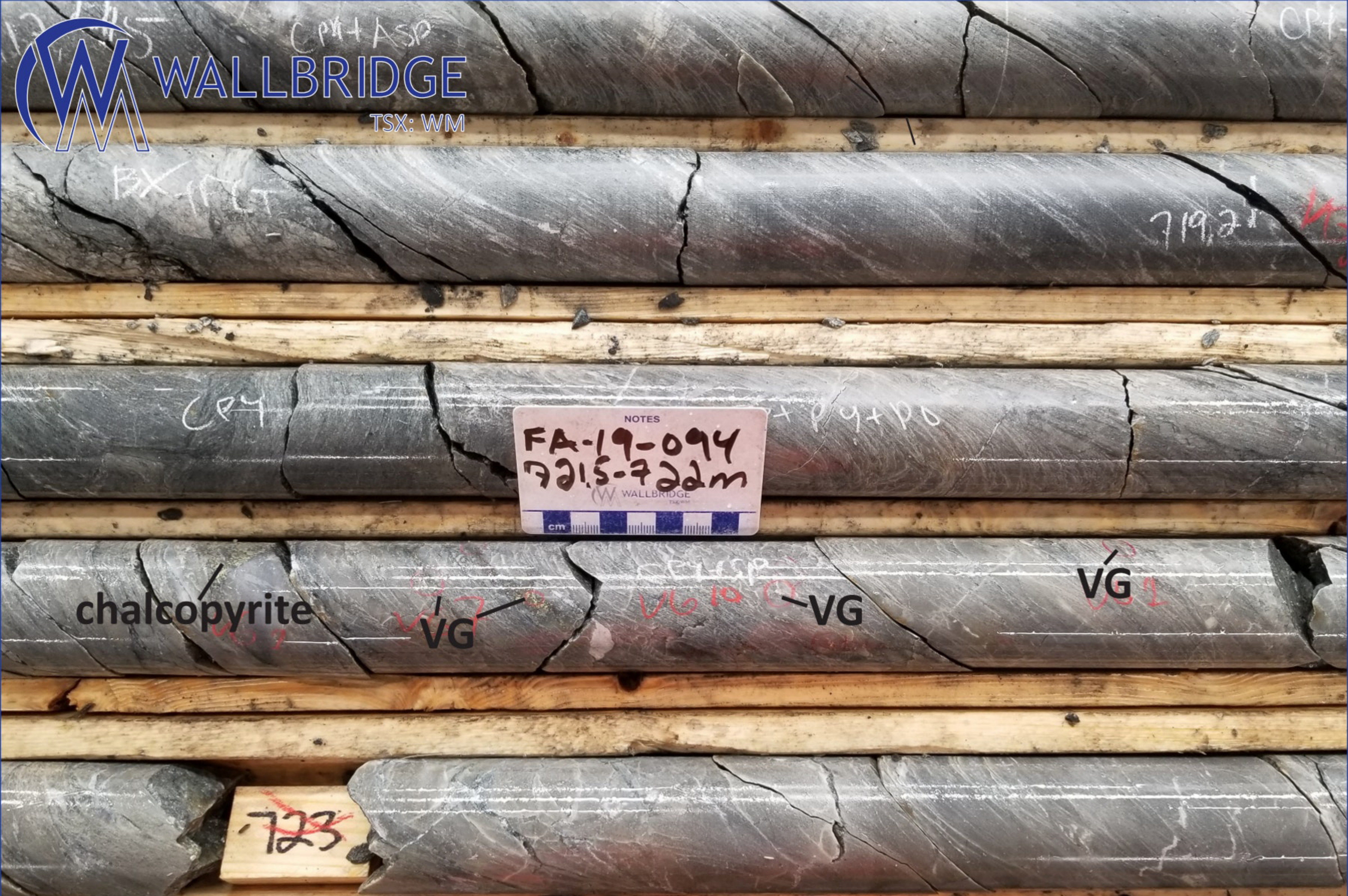
Fenelon Gold - Drill Hole FA-19-094 (721.5-722.0 m): Tabasco Zone Approximately 13-metre core length (717-730 m) with abundant sulfide and visible gold
