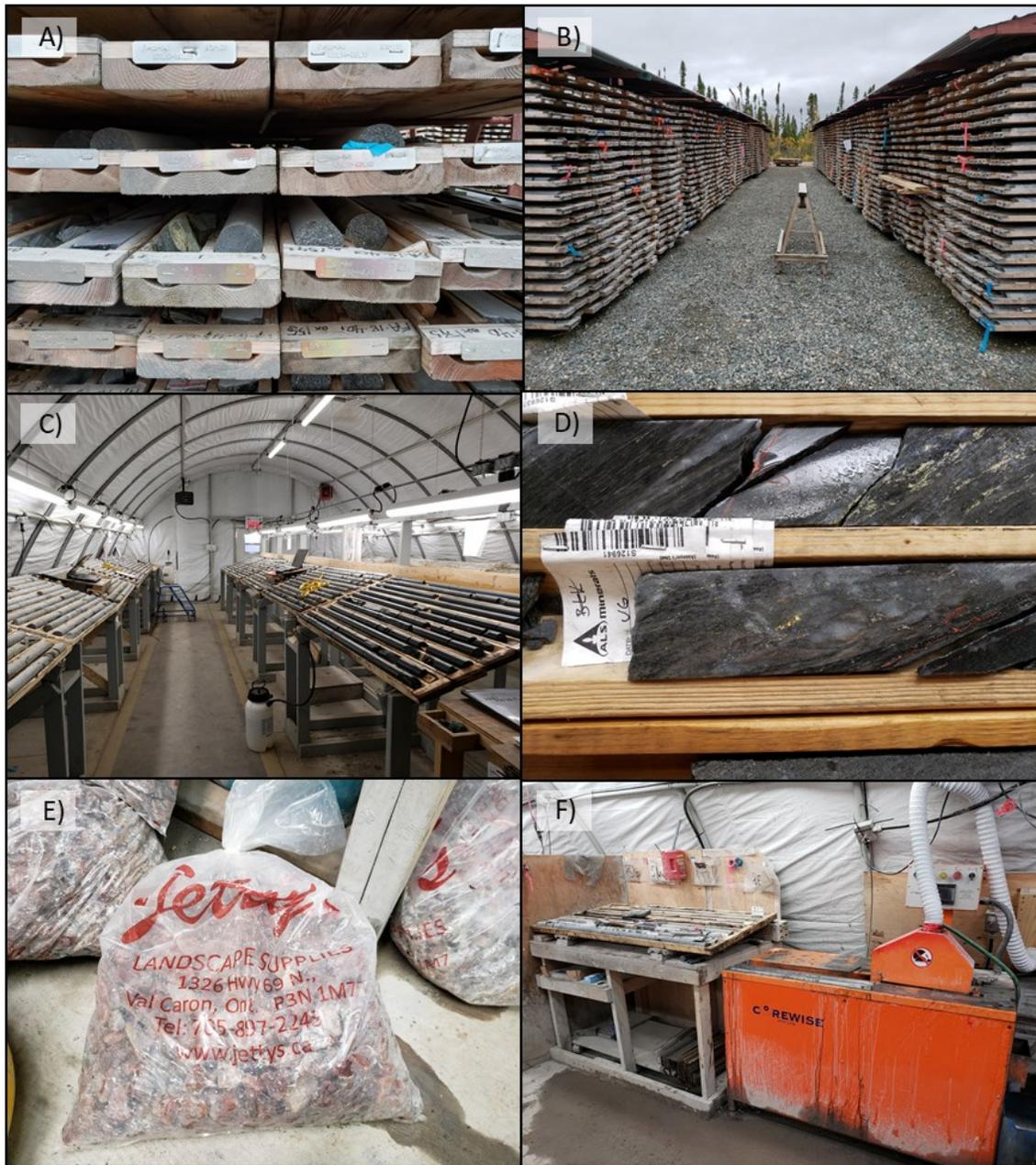
A) Proper labelling of the drill core boxes; B) Outdoor core storage; C) Logging facility; D) Sample tags stapled in core boxes showing length and depth of the sample; E) Barren material used as blanks; F) Sawing facilities. (October, 2019)
