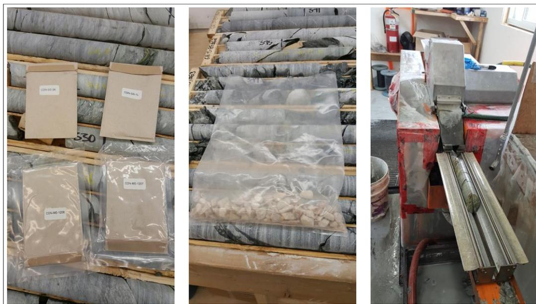
**Figure 12.8 – Photos of the different standards, the commercially crushed material used as blanks, and the area dedicated for sawing and preparing samples for the laboratory**
