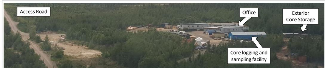
**Figure 12.1 – Photo of the office, core logging and sampling facility, and the outdoor core storage area. Photo taken during the site visit**
