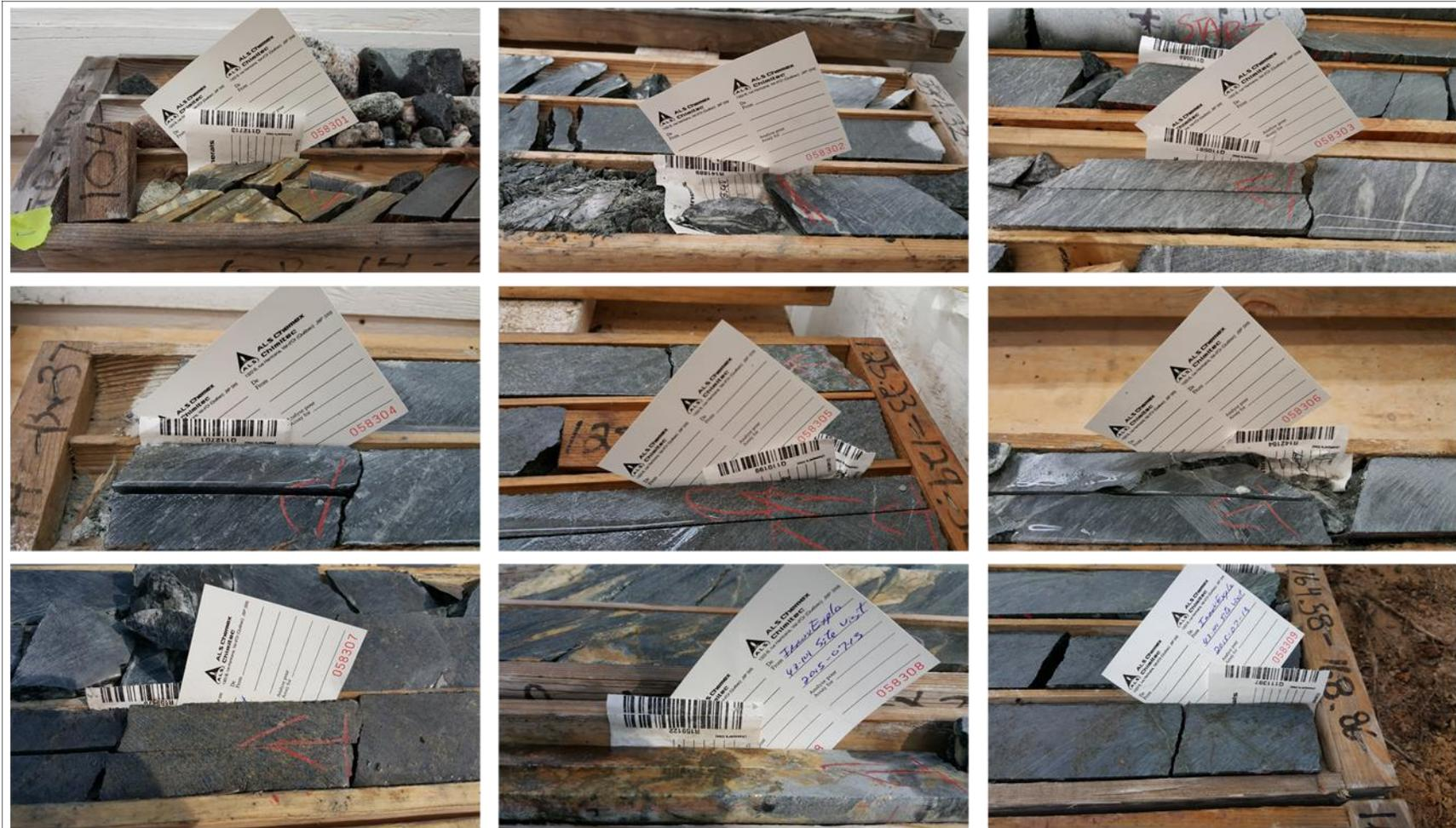
**Figure 12.9 – Views of some of the core reviewed at the core storage facilities visited by the author. These are the nine samples that were re-assayed as part of the data verification process. Note that some of the original tags showing in the photos identify a standard or a blank, thus the tags for the original core samples are found under these QA/QC tags.**
